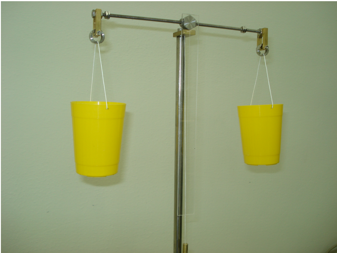
Fig. 1.6.4 Symmetric balance used to exemplify the notion of physical quantity with the example mass.
